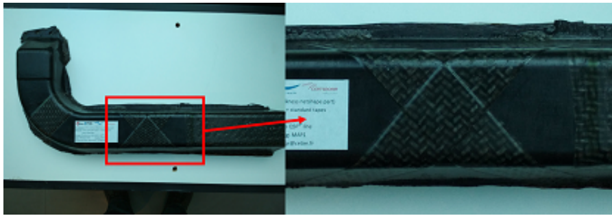
Fig. 19.: Final position of woven prepreg patches : experiments
