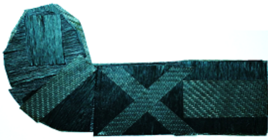
Fig. 1.: Flat 2D stack of prepregs before QSP®
