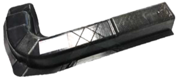
Fig. 2.: Thermoformed 3D final shape after QSP®
